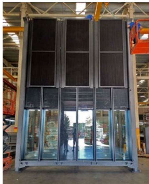
Mock-up image of the photovoltaic glass to be implemented in the tower, designed by the architecture firm Mecanoo.
